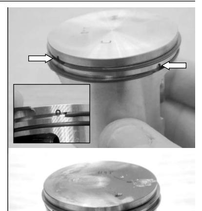
13.15 Install one wrist pin retaining clip.
